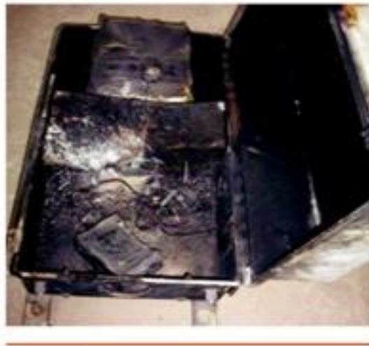
Fig. 4.29 Burnt Energy Meter Due to Short Circuit
